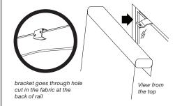
5. Secure the shade to the brackets by tightening the ½" set-screws.
