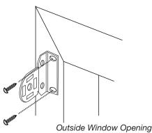
Mark the screw locations with a pencil – pre-drill the screw holes using a 5/64" drill bit.
