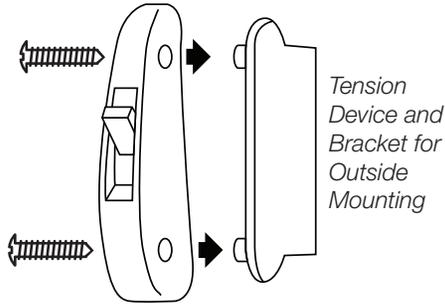
Tension Device and Bracket for Outside Mounting
