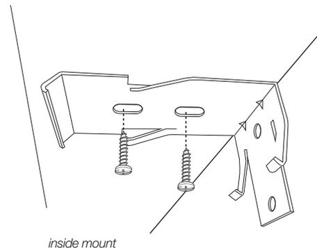
The other bracket(s) should be spaced evenly between the two outermost brackets.
